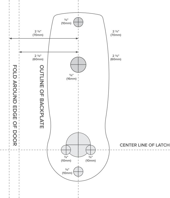
Fix this template in position on the locker door to ensure holes are drilled accurately.
