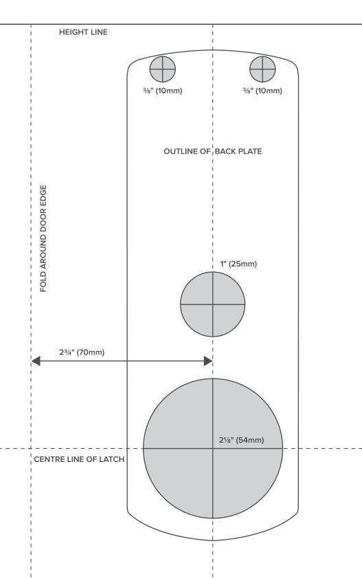
Pix this template in position on the locker door to ensure holes are drilled accurately.
