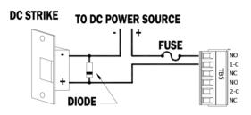
The AUX power output may be used to power the strike if 12Vdc is required and the power rating is not exceeded. An external power supply may be required
